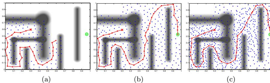
**Fig. 2.** Static Puddle World: (a) and (b) shows the graph at the beginning of learning and when the agent has found the goal for the first time. (c) results from further optimization of the graph. The red line indicates the best known policy to the target.
