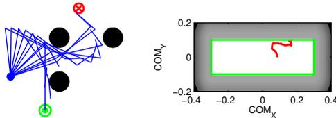
**Fig. 4.** Arm reaching task with stability constraints. Left: Solution trajectory found by our algorithm. The agent must reach the goal region (red) from the starting position (green), avoiding the obstacles. Right: Trajectory of the CoM of the robot (red) inside the neutral zone (green).
