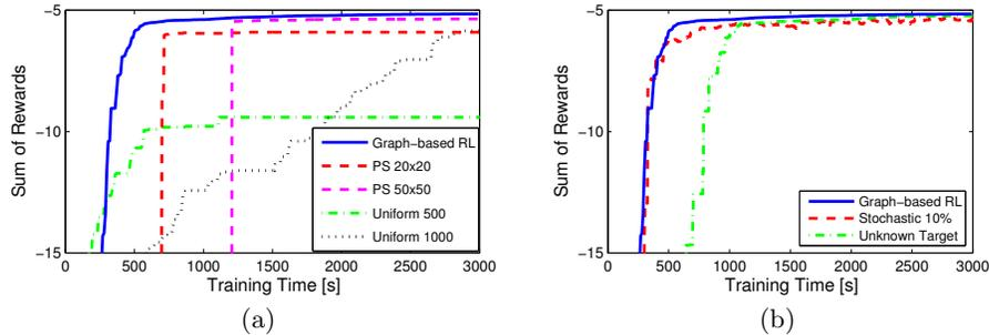
**Fig. 3.** Learning performance on static puddle world from Figure 2. (a) Comparison of RL with adaptive state graphs to prioritized sweeping (PS), and greedy search on uniformly sampled nodes (Uniform) with different discretization densities. (b) Influence of stochasticity (10% movement noise) and unknown target states on performance of graph-based RL. (Average over 10 trials.)
