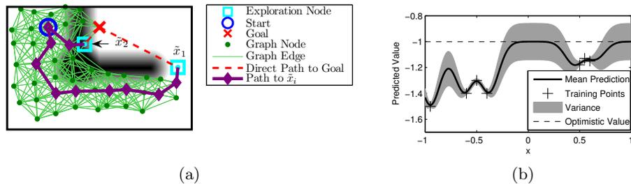
**Fig. 1.** (a) Illustration of the exploration process. Exploration node  $\tilde{x}_1$  is preferred over  $\tilde{x}_2$ , because the reward to reach  $\tilde{x}_2$  is strongly negative. (b) Illustration of value prediction with Gaussian processes on an artificial 1-D dataset. The prediction approaches the optimistic value and has larger variance for points that are farther away from training points.
